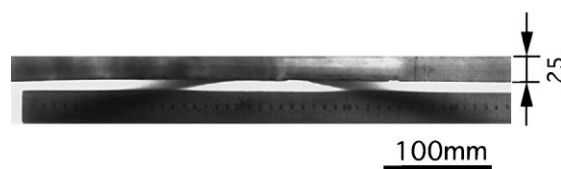
Fig. 3. A sheet formed by electrically heated powder rolling.
